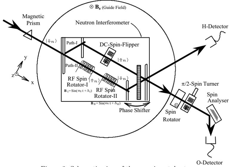
Figure 3: Schematic view of the experimental setup.
